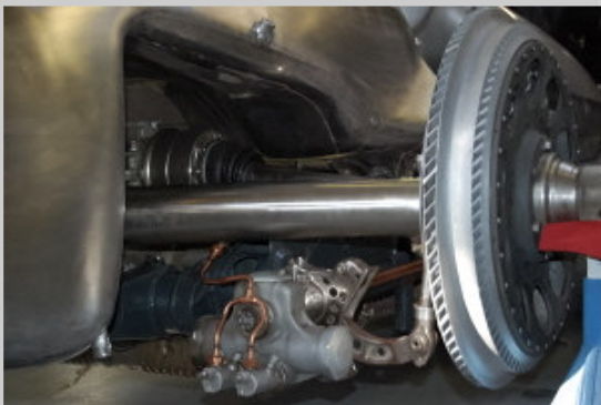
Jet turbine-like cooling of drum brakes and hydraulically adjustable anti-sway bars (bottom center) Photos by Swenson
