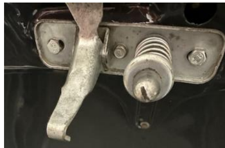
John's latch bolt assembly with slot at end of bolt.
