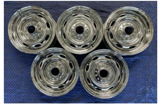
15x4.5" Rudge Knock-Off Wheels and Brake Drums for Porsche 356
