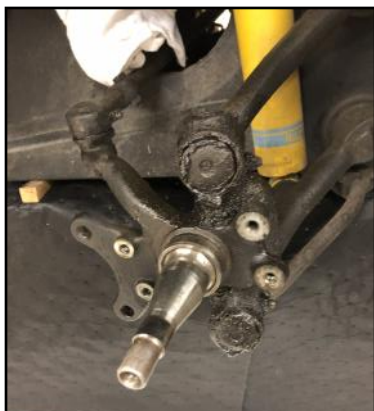
Left and right- Before and after cleaning on of the front spindles.
