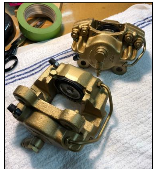
Rebuilt and refinished front calipers.
