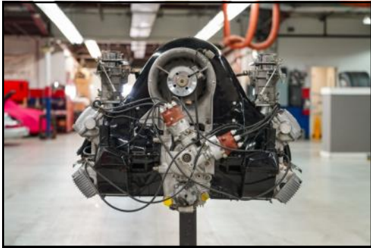
Porsche Fuhrmann Four-Cam Engine
